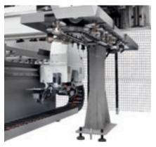
22- or 33-place chain magazine with fixed floor position, available with single or dual configuration.
