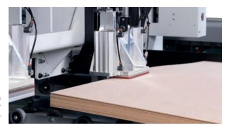
The gripper loading system allows both single and multiple panels to be safely and accurately loaded into the machine, significantly increasing productivity.
