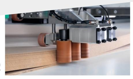
**Rollers, for aligning** the individual panel or a stack of panels, ensure maximum load precision.
